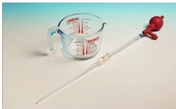
Figure 4 A bulb pipette has less resolution than a measuring jug but is more accurate at measuring 25 cm 3 of liquid at 25 °C.
